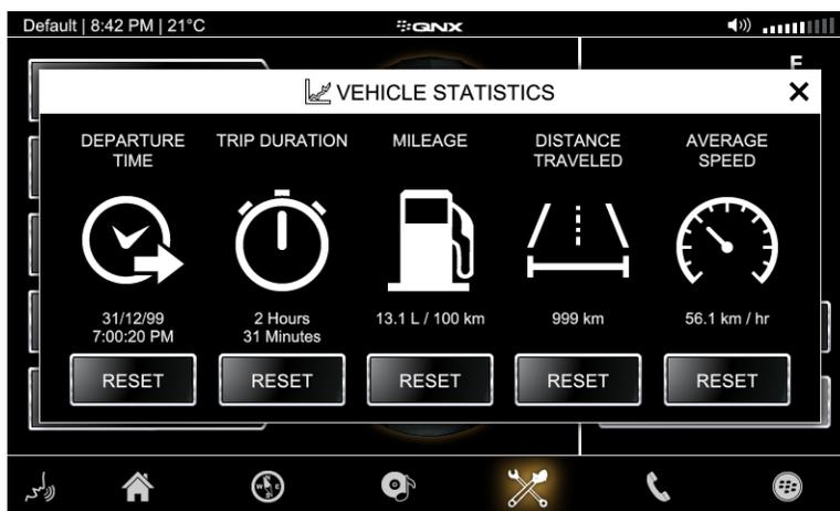
When you tap the **RESET** buttons, the data is reset to zero for each measurement except DEPARTURE TIME—this value is reset to the current system time.
