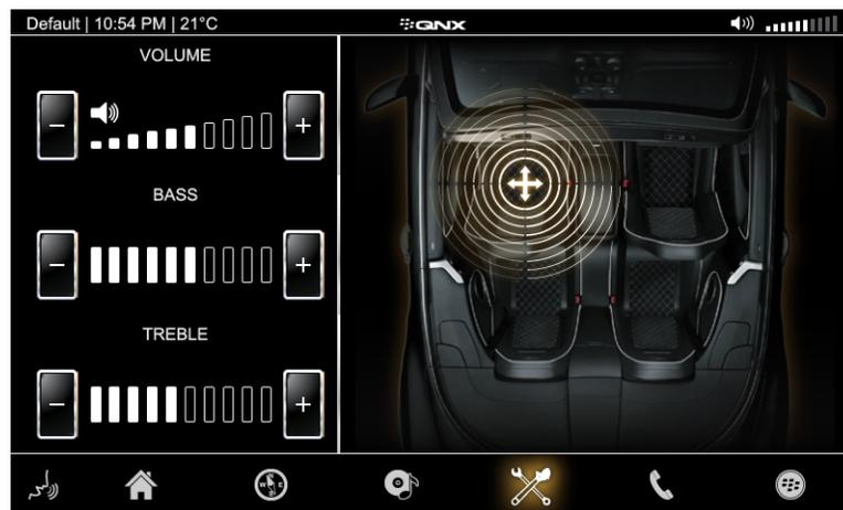
The **Audio Control** feature is the only place in the HMI where you can set the volume—there's no separate app for controlling the volume of audio playback. The **Bass**, **Treble**, and balance controls are active but not functional.
